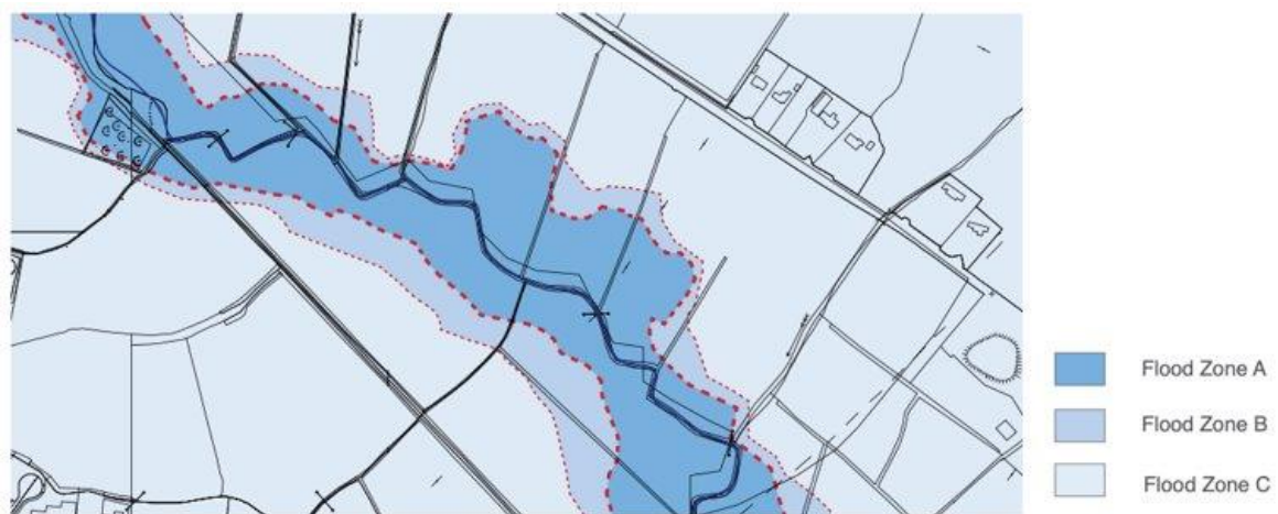
Figure 2: Indicative Flood zone map from (Dept of Housing, Local Government and Heritage, 2009)
